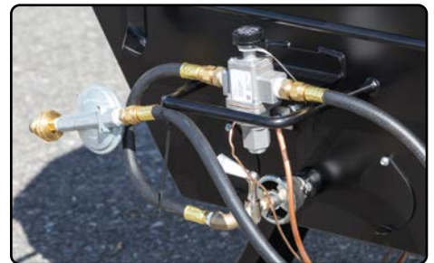
Gas Safety Valve
