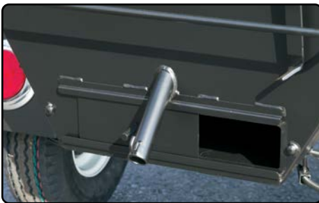
Bottom Damper and Drip Tube
