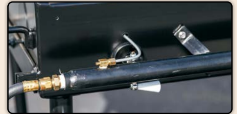
Gas Manifold With Cover Removed
